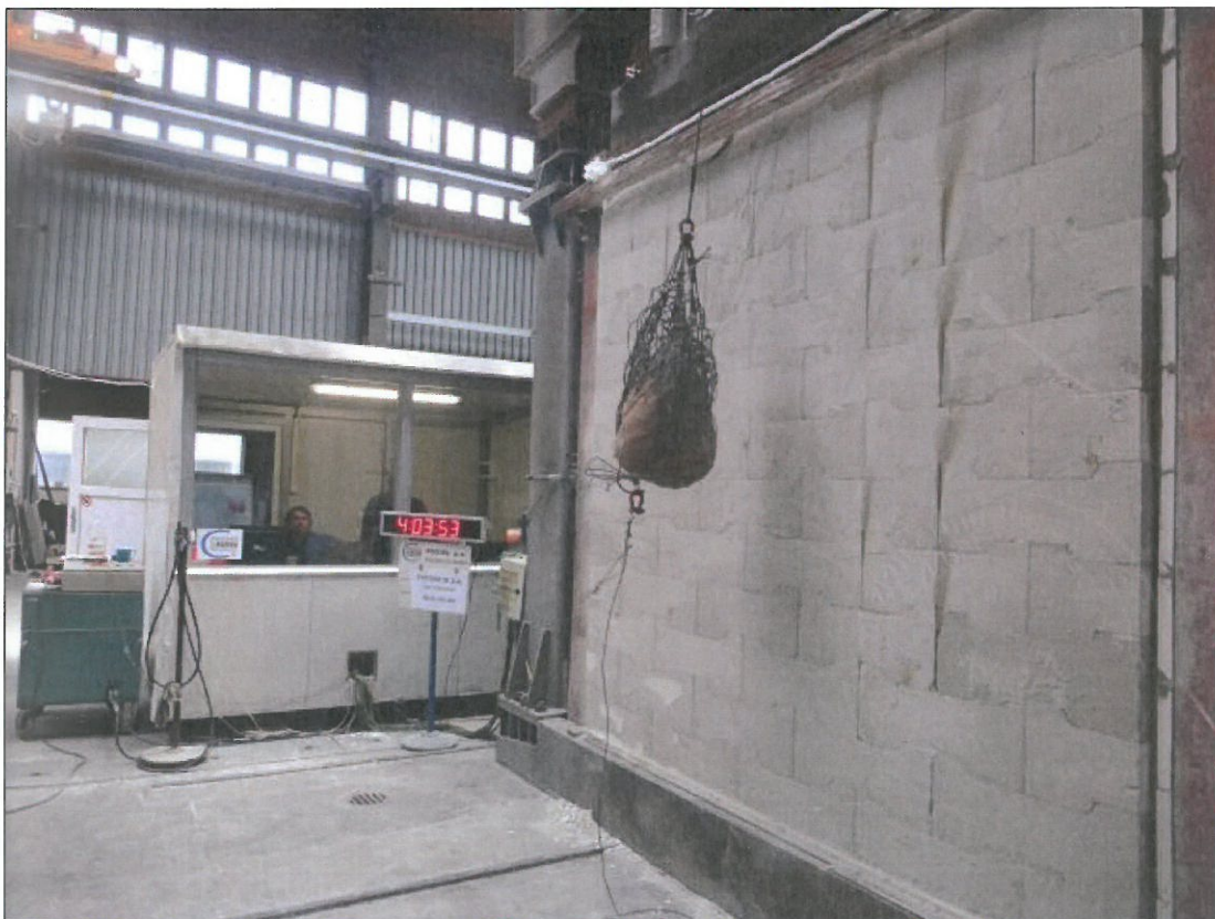
244 th test minute - view of UF after the second impact, removal of the test load
