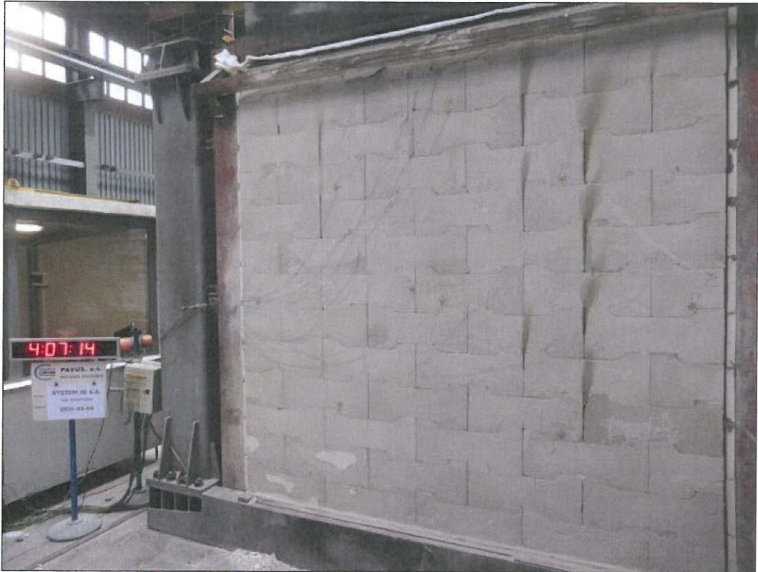
248 th test minute - view of UF after the third impact
